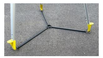
2. Detach elastic loop from tripod star leg, double the loop over and fit onto the tripod leg as far up the yellow spiked foot as you can, repeat on other two legs.
