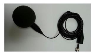
3. Finally, push the foam All Weather Windscreen onto the microphone so it meets the boot. The microphone is now ready to be fitted to the microphone clip on the boom arm
