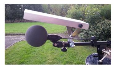
Microphone shown with the Weather Shield fitted. Note slight upward angle of the microphone.
